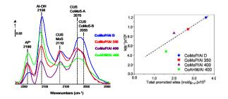
The number of Co-promoted sites in  $CoMoP/Al_2O_3$  HDS catalyst prepared with  $Co_{7/2}PMo_{12}O_{40}$  depends on the pretreatment given to the catalyst before its activation (sulfidation). Two different types of promoted CoMoS sites with different HDS intrinsic activities seem to co-exist in the sulfided catalyst.
