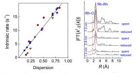
The intrinsic rate for steam methane reforming of Rh increases linearly with metal dispersion independent of the support (CeO<sub>2</sub>, CeZrO<sub>2</sub>, ZrO<sub>2</sub>, ZrO<sub>2</sub>, SiO<sub>2</sub>) when corrected for the amount of non-nonreducible Rh.  $CH_4$  activation is rate limiting under typical steam reforming conditions. At a temperature of 500 °C catalysts containing very small Rh metal particles deactivate due to oxidation of the metal phase.
