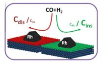
As ascertained using highly dispersed model  $Rh/M@Al_2O_3$  catalysts, the selectivity pattern in the synthesis of oxygenates from synthesis gas is dictated by the electron-withdrawing/donating power (Lewis acidity/basicity) of the underlying metal oxide promoter.
