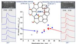
Internal framework defects are crucial for the deactivation behaviour of the ZSM-5 catalysts in the conversion of methanol to hydrocarbons. While the activity is related to the acid site density, the deactivation rate correlates with the measured intensity ratio of the IR bands for internal silanols at 3726 cm<sup>-1</sup> and for external silanol groups at 3745 cm<sup>-1</sup> ( $I_{3726}/I_{3745}$ ).
