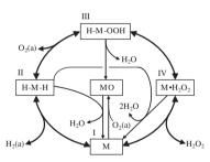
Kinetic analyses of the direct  $H_2O_2$  synthesis from  $H_2$  and  $O_2$  and the  $H_2O_2$  decomposition on Pd/C catalyst in water containing  $H^+$  and  $Br^-$  ions and adsorption measurement of  $Br^-$  ion on the catalyst proposed a hydride-hydroperoxy species H-M-OOH (M represents the metal surface) to be the key intermediate in the  $H_2O_2$  formation, the direct  $H_2O$  formation, and the  $H_2O_2$  decomposition.
